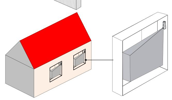
Example of installation on fixtures. The height of the detector must always be calculated with respect to the reference plane which must not be more than 2.1 m
