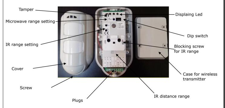
Triple technology outdoor detector made with double infrared sensor and microwave. Adjustment of microwave flow by trimmer placed inside.
