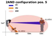
Using the bracket you can change the height of fixing
