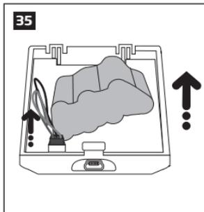
5. Pull up the battery (unstick it), disconnect the battery's cable and pull the battery out
