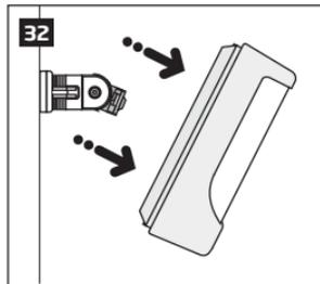
3. Remove the device from its holder.
