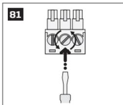
3. Connect **BELL** wire (usually - red) of the wired bell/siren to **BELL+** terminal, while the **GND** (usually - black) wire to **BELL - / COM** terminal.
