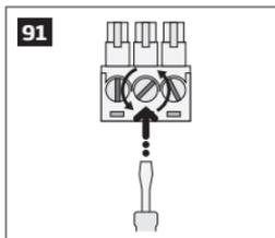
3. Connect the 5.6k $\Omega$  nominal resistor, supplied with your PITBULL ALARM PRO (or PITBULL ALARM PRO -3G) system, across **BELL- / COM** and **ZZ** terminal in parallel to the connected wires of the detection device.
