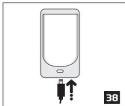
Plug the mini-USB connector into the device.
