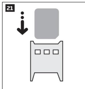
Then insert the SIM card into the slot. Insert SIM card so that gold contacts are face down.
