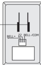
1. Alarm system's holder for fixing on the wall
