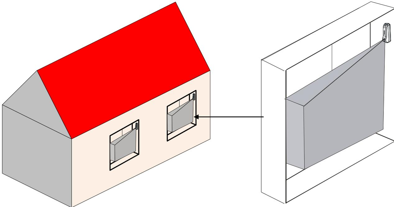
Example of installation on fixtures. The height of the detector must always be calculated with respect to the reference plane which must not be more than 2.1 m
