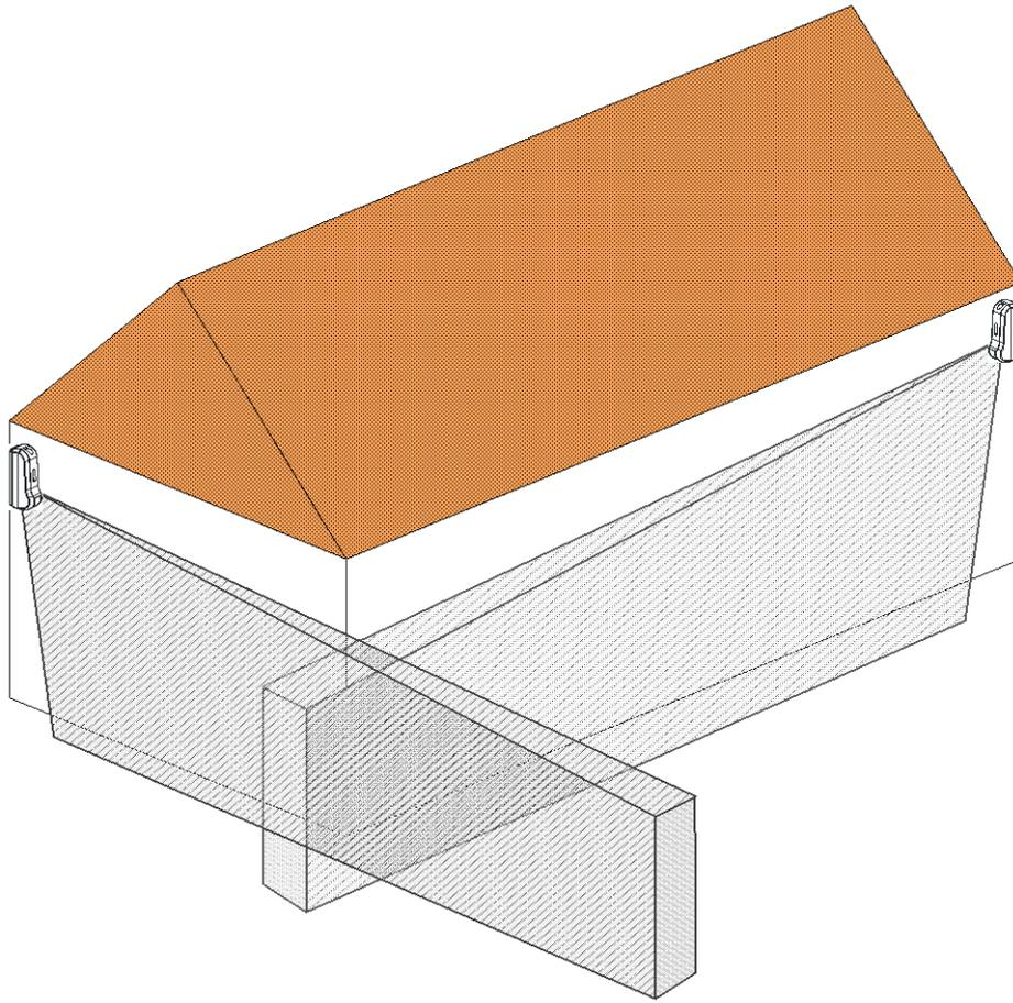
Example of installation to protect walls. Install at approximately 2.1 m in height. It can also be installed on the upper floors still at 2.1 m with a horizontal plane at least 1.5 m wide as a reference for the entire detection length (for example, balconies, frames). Make sure there are no obstacles that prevent detection (gutters, blinds, etc)
